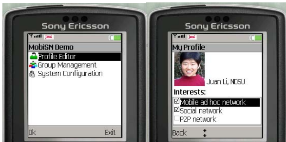
Figure 3. MobiSN prototype running on the SonyEricsson_K750.
